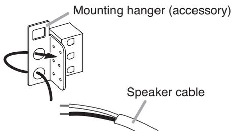
**Step 4.** Connect the speaker cable to the screw terminal.
