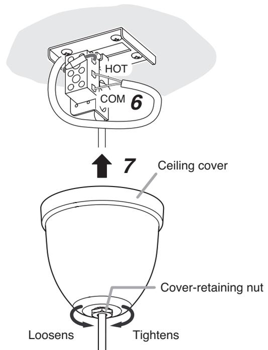
**Step 7.** Push the ceiling cover, slipped over the connected cables, onto the ceiling surface, then tighten the cover-retaining nut using a 17 mm (0.67") hex wrench.
