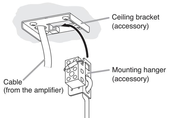
**Step 6.** Connect the cable (from the amplifier) to the screw terminal.
